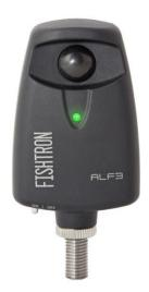
The portable FISHTRON ALF3 detector is designed for fishermen to detect the movement of people in a fishing area, equipment, parked car or other property of a fisherman. Integrated sensors respond to motion and wirelessly transmit information to the receiver that the fisherman has with him.
